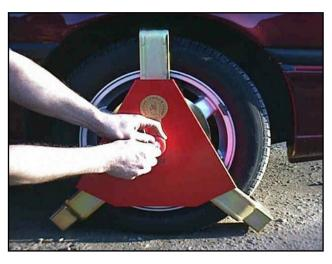
11. Press thumb against red cap, push in key and rotate 1/4 turn anti-clockwise to UNLOCK. Now place cover plate (part No.11) so that lock engages with hollow nut and rotate key 1/4 turn clockwise to LOCK and release key.
