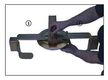
4. Remove hollow nut from inside cover plate and screw on finger tight but still allowing arms to slide freely. Please ensure that the recess on back of nut is located into hole in large spring washer. Now fit M10 coach bolt, bushes and nuts as shown, to bottom arms No. 1. These can be tightened by using spanner (14). Fit rubber disc to rear of steel disc.
