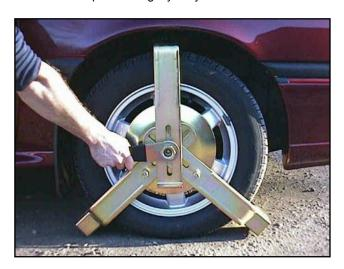
Using spanner provided tighten nut in a clockwise direction until it locks up solid. NB. When removing clamp reverse steps 10 to 6.
