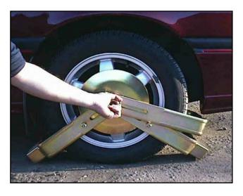
With left hand lift nut and disc assembly to centre wheel.
