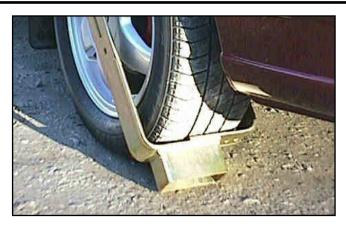
**2a.** Make up each arm and arm return to width of tyre (allow for width of disc, part no. 6).
