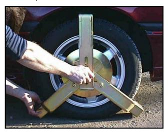
**9.** At this point hold up nut with right hand and pull left wheel clamp arm in tightly to tyre. Now hand tighten nut.
