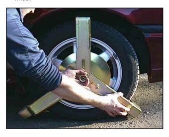
**8.** Still holding up nut with left hand, pull the right wheel clamp arm in tightly to tyre.
