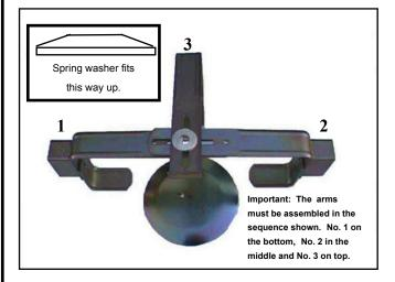
3. Position lower arms as shown and lay top arm on top. Place in position spring washer, push square head of M12 x 40mm coach bolt into round disc. (Tap with hammer if tight fit) until dome head touches disc. Offer up round disc to lower arm, ensure that the pressed dimple on the disc locates securely in slot in arm, this is to prevent turning.
